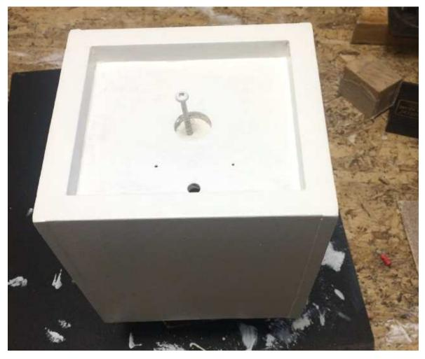
When the paint on the box had dried I reinstalled the speaker and the terminal strip, wired it all together, threw in some insulation to cut out any boomyness and it was done.
