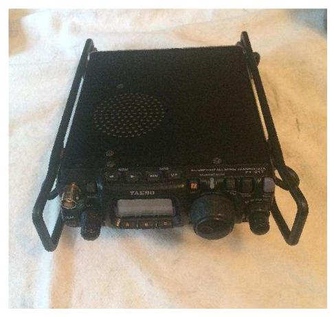
My sole interest is HF CW and the FT-817 did not have the optional CW filter which I soon found to be made of pure unobtainium. BUT! A Timewave DSP-9 was found in the back of the closet and it does a very cost effective job of subbing for the missing CW filter.
