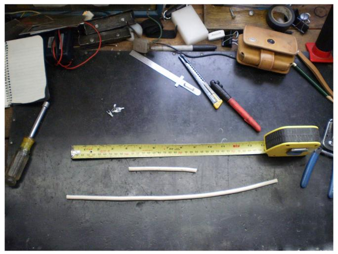
I trimmed the pieces to appropriate length, and put lugs on one end of each piece to accommodate putting them under the nuts that hold the elements in place. I soldered the lugs on, in case of a mistake, I could remove them, and start over (usually happens). After installing the harness, it was time to find a piece of pipe to fit the cap and use as a base.
