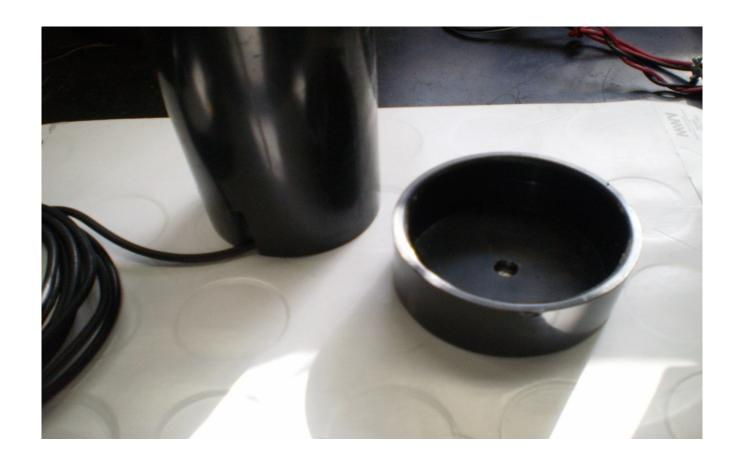
After dry fitting it all together, I hooked it up to my receiver, and noticed a considerable improvement in signal strength. Apparently, you can add a reflector made from chicken wire (all us old timers remember what that is, don't we...) to add more gain. Also, if you notice the hole in the bottom of the base cap, that is to mount it on a tripod to aim it south at the satellite belt.
